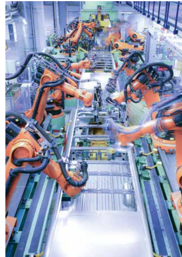
Complex welding system with ARC module for the MIG welding process
