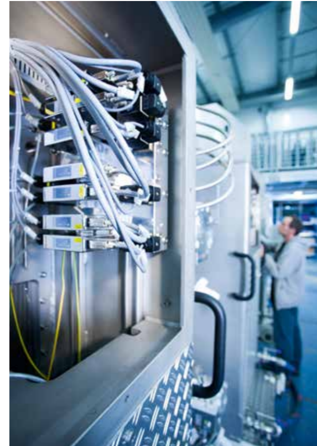
Coating system with fully automated gas control
