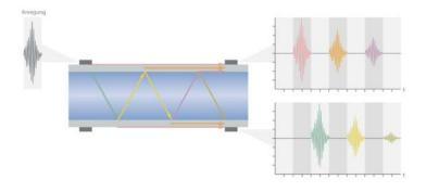
Caption 3: The Surface Acoustic Wave (SAW) technology on which FLOWave is based uses wave propagation such as that which occurs in seismic activities.
